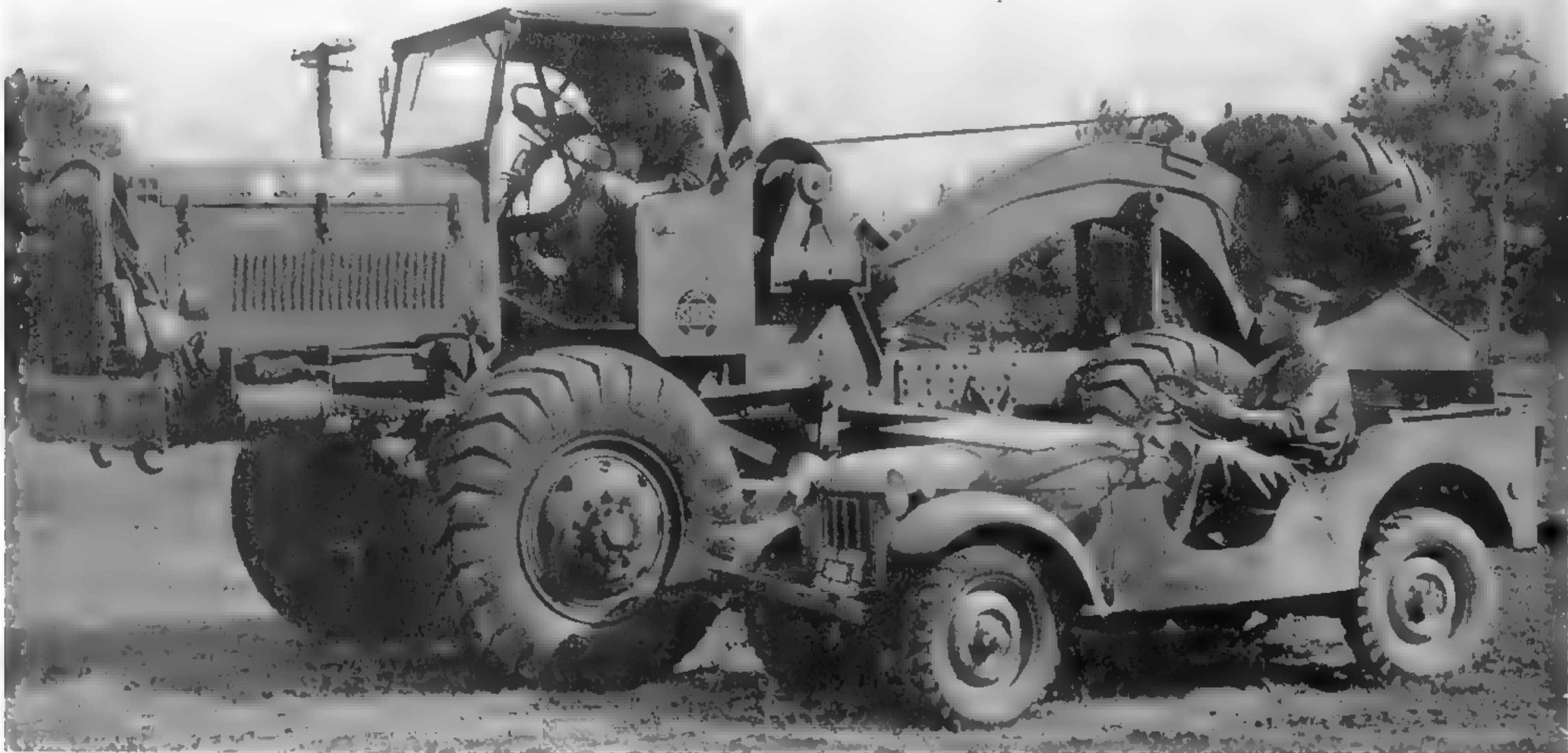
Shown here is arguably the original Jeep, the prototype Bantam Reconnaissance Car. Notice the scalloped cutouts for crew access and the curved fenders and separate protruding headlights without brush guards. All these features that were eliminated when the first 75 pre-production units were built. The massive 4x4 beside it is a 5-ton prototype artillery tractor built by Oshkosh. (U.S. Army photo)
